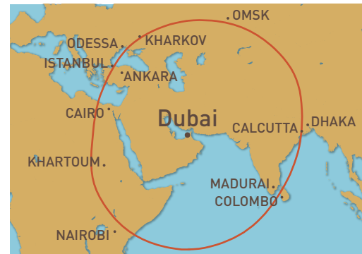
Depicted range is approximate. Map distortions prevent exact range representation. Assumptions: NBAA IFR Reserves (100 nm), ISA Enroute, 85% Boeing Winds, Great Circle Distances, High-Speed Cruise, two crew, four passengers.
